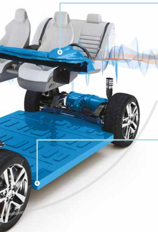
Battery insulation/Transmission undertray
