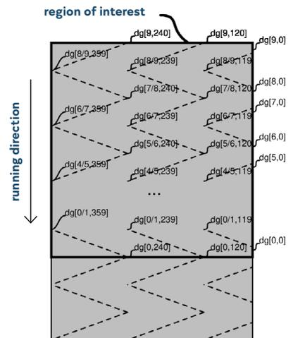
Another key advantage of using this scanning system is the continuous measurement taken not only in machine direction, but also in cross direction. This is thanks to the traversing movement of the Marveloc-Curtain frame which carries the measuring sensors (Fig. 1).
